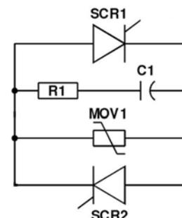
The typical failure mode of the circuit is the explosion of the MOV. MOVs
