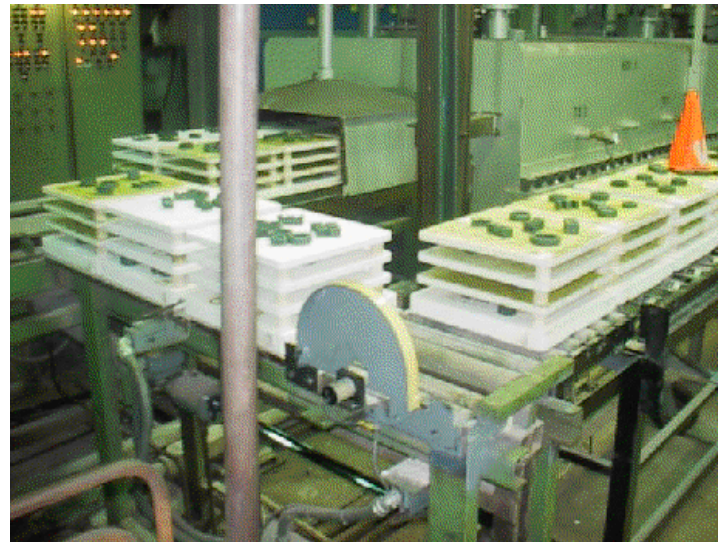
Parts entering Double Wide Kiln
